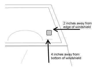
NOTE: The AVI Tag must be installed with the <u>blank side facing the outside</u> of the vehicle, toward the AVI Reader.
